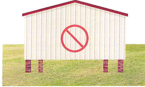
No Installs on Stacked Blocks
