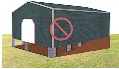
No Installs on Unlevel Land
